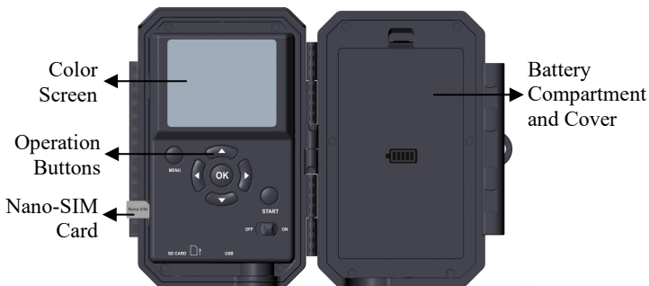
Figure 4: Inside View and Preinstalled SIM card
