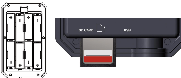
Figure 5: Installation of batteries and SD card
