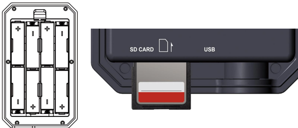
Figure 5: Installation of batteries and SD card
