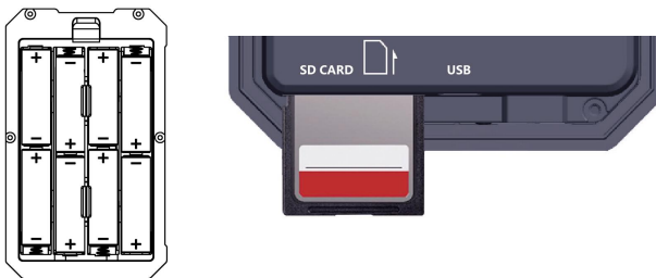
Figure 5: Installation of batteries and SD card
