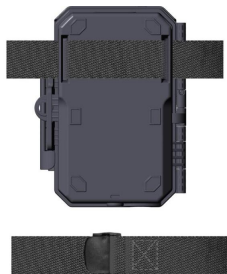
Figure 17: Mounting the Camera
